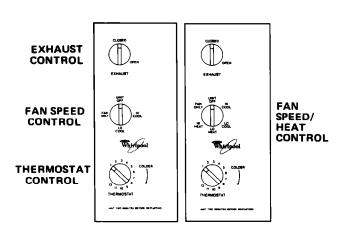
Be sure air conditioner is OFF before plugging it in. NOTE: Exhaust Control not available on Models ACE864 and ACW864.
